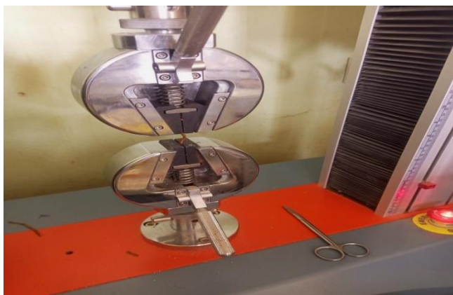
Figure I: The Universal Testing Machine used to measure the tensile strength of the experimental samples
